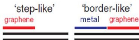
Figure 3.1 Scheme for visualization of the difference between border-like and step-like edges. Figure adapted from 264 .
