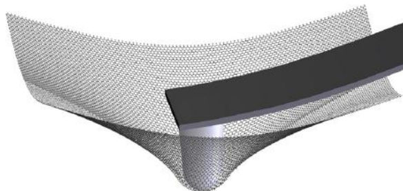
Figure 2.7 A representation of a diamond tip with a two nanometer radius indenting into a single atomic sheet of graphene. Figure extracted from 22 .
